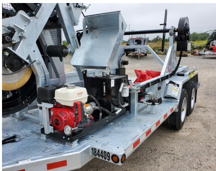
HYDRAULIC POWER PACK AND TAKE UP UPGRADE
